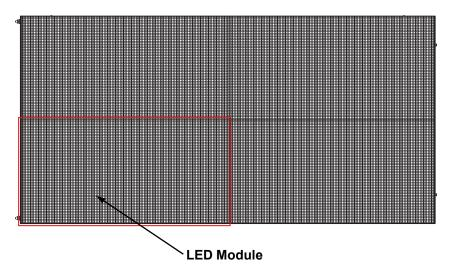
Each pixel is 1 tri-color LED. The following table provides the pixels per panel in each F2. For detailed specifications, refer to the Technical Specifications table at the end of this User Manual.
