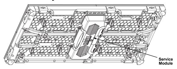
The F2 service module can be accessed and serviced from either the front of the panel or the rear of the panel at any time, so panels can be serviced when access to either the front or the rear is restricted or impossible. Follow the instructions below to access the F2 service module from the front of the panel:
