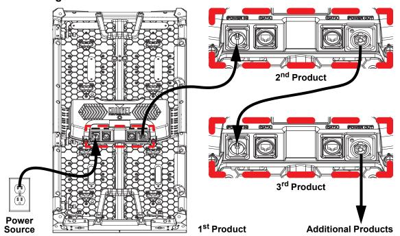
All F2 panels support power linking. Refer to the following table for specifications on each panel.
