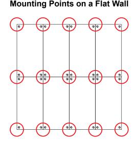
At least 1 mounting point for every junction (circled above) must be secured, including outside edges and corners
