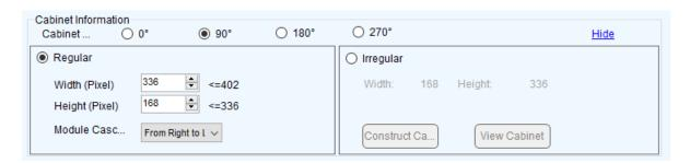
14. Select either 90° or 270° to rotate the video within the connected panels.
